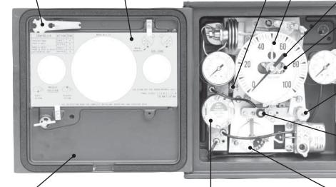
CASE: Cast aluminum with dust ledge and deep weatherproof gaskets, captive stainless hinge pins and latch shaft, rectangular glass. Optional gas-tight construction with case tapped for 1/2" pipe vent. For high-pressure applications, shatter-proof glass and blowout grommets are available. Anodize is available for maximizing corrosion resistance.
