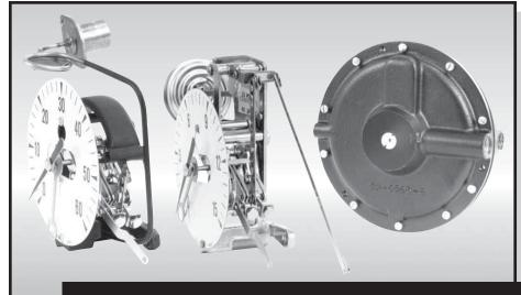
LEFT, "C" TYPE BOURDON TUBES; CENTER, DIAPHRAGM ELEMENTS; RIGHT, SLACK DIAPHRAGM
