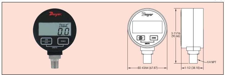
The Series DPGW is the only economic digital pressure gage for liquids with the ability to select engineering units on the market. With its 1% accuracy and digital push-button zero, the DPGW is the perfect choice for digitally monitoring the pressures of compatible liquids and gases.
